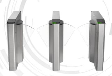
The DS-K3Y220LX series swing barrier with 4 pairs of IR lights is designed to detect unauthorized entrance or exit. By adopting the flap barrier integratedly with the access control system, person should authenticate to pass through the lane via presenting IC or ID card, scanning QR code, etc. It is widely used in factories, construction sites, residences, etc.
