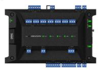
The access controller supports web configuration, which is no need to install software on a PC. By connecting with access modules via RS-485, it can extend to control up to 126 doors, which is suitable for the scenarios of subways, airports, banks, large groups and other industry projects.
