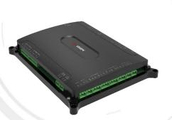
DS-K2601T access controller (main board) is designed with latest structure with TCP/IP and RS485 communication interface. The communication data is encrypted to improve the security of system. The controller also supports offline operation.
