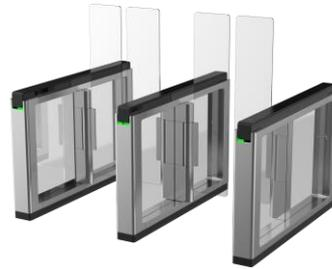
The swing barrier with two barriers and 24 pairs of IR lights is designed to detect unauthorized entrance or exit. By adopting the swing barrier integrated with the access control system, person should authenticate to pass through the lane via swiping IC or ID card, scanning QR code, etc. It is widely used in high-end offices, government buildings, hotels, airports, etc.
